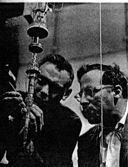
Figure 3 Scientists checking a helium refrigerator developed for laboratory use to maintain temperatures as low as 0.04° above absolute zero. When in use the instrument is enclosed in a vacuum chamber.
