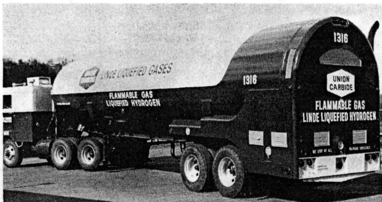
Figure 17 Liquid hydrogen transport truck. This 13,400-gallon Dewar, largest mobile unit in the United States, meets all regulations for safe highway transport of liquid hydrogen. It is vacuum-insulated but to conserve space and weight only a few inches of "superinsulation" are used in the vacuum space.
